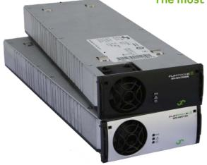
The combination of innovative design, efficiency and reliability makes the Flatpack2 HE stand out. With efficiency up to 96.2%, the losses have been reduced by 50% compared to the current industry standard. Compared to older technologies with even poorer efficiency an investment in a Flatpack2 HE system is repaid in a few years by the reduced operating cost.
